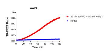
Activity Assay of WWP2. 25 nM WWP2 + 50 nM Ndfip1 were tested in a TR-FRET assay for 120 minutes and showed a robust Signal to Background ratio.
